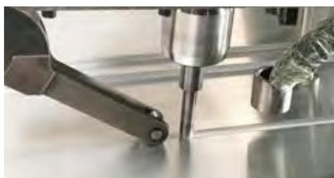
Joining the metal using the FSW technology
